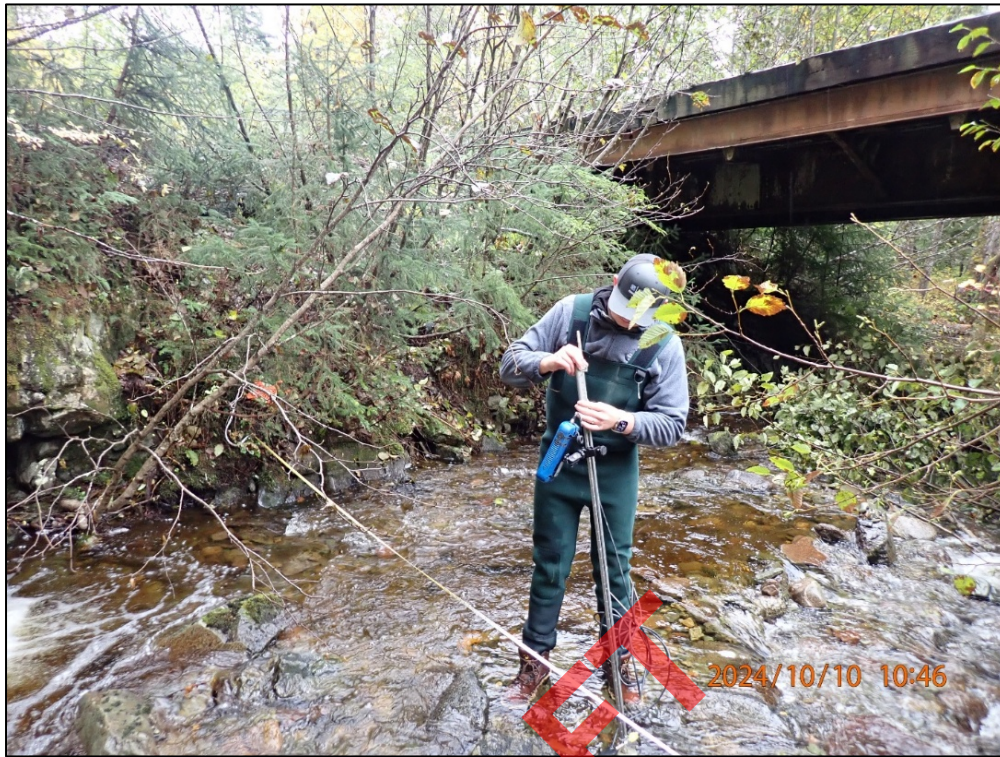
Figure 5: Measurement of streamflow conducted at the time of the site visit on October 10 th , 2024.
